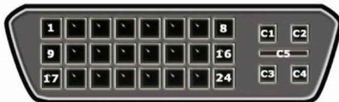
Figure 19: DVI-I Signal Pins
